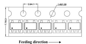
2. Carrier Tape & Reel specification for packages
