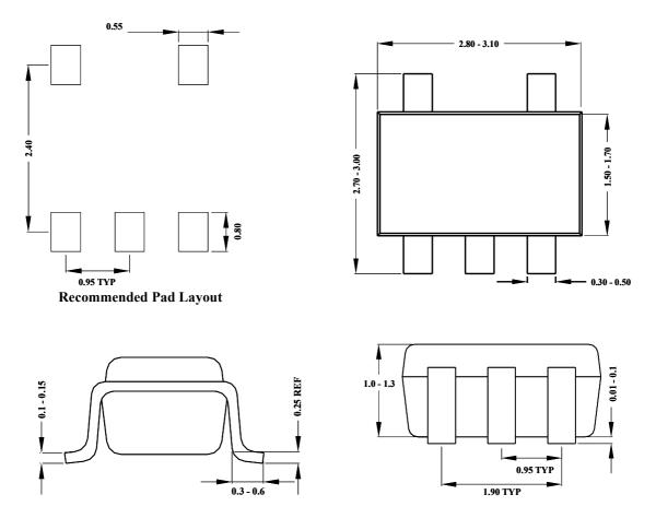
Notes: All dimensions are in millimeters. All dimensions don't include mold flash & metal burr.
