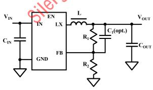
Figure 1. Schematic Diagram
