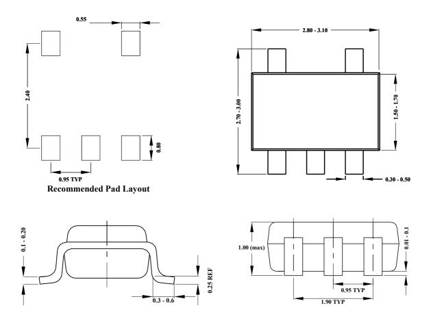
Notes: All dimensions are in millimeters. All dimensions don't include mold flash & metal burr.
